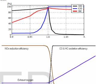
A dual bed catalyst depends on air injection to provide the oxygen to clean up CO & HC when the mixture is rich. Air is only injected into the rear bed. Many cars do not have air injection. Without air injection and a slightly rich mixture these cars must depend on something else to manage the oxygen in the catalytic converter.
